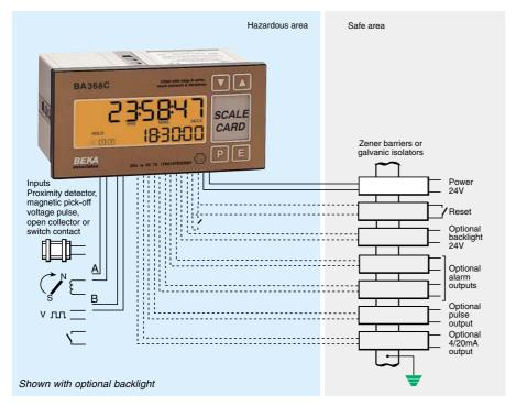
The BA368C is an intrinsically safe multi-function instrument which may be programmed to perform a host of counting and timing functions. Easy to use menus allow the instrument to be configured as a counter, timer, tachometer or as a clock. Both of the inputs will operate from 2-wire proximity detectors, switch contacts, magnetic pick-offs, open collector or voltage pulses. Optional alarm/control outputs further extend the many applications.
